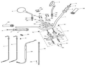
Handlebars, top yoke, cables & mirrors
