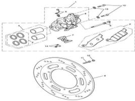
Front brake caliper & discs
